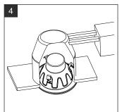
4. Insert recessed downlight into fixture housing. Use clips to keep in place. Carefully route wires into fixture and push recessed kit up flush to ceiling surface.
