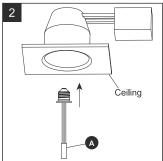
2. Screw adaptor (A) into socket in recessed housing.
