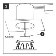
3. Plug base cable connector on adaptor (A) into lamp (B)
