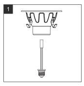
1. Make sure the power is turned off at the source to the recessed housing(s) where the fixture(s) will be installed.
