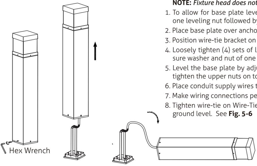
**NOTE:** Fixture head does not need to be removed from bollard pole during installation.
