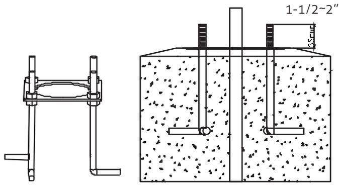
**NOTE:** Anchor bolts, template, and wire-tie bracket are attached to base plate for shipping.
