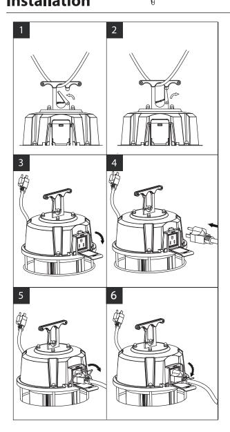
**STEP 1.** Place the work light up to the hanging hardware, push the latch of the carabiner clip against the hanging hardware until it opens (Fig 1) and captures the hardware (Fig 2).
