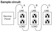
Placing the GFCI in position A will also provide protection to " load side "receptacles/outlets B and C. On the other hand, placing the GFCI in position C will not provide protection to receptacles/outlets A,or B .Remember that receptacles /outlets A, B and C can be in different rooms.
